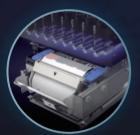
An easy-to-replace cloth wiper roll continuously wipes the printhead nozzles clean to remove fluff that can cause nozzle clogging.
